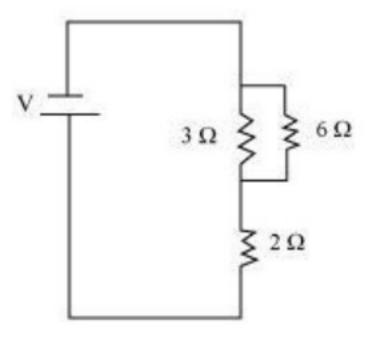
This equivalent resistor of resistance 2  $\Omega$  is connected to a 2  $\Omega$  resistor in series.
