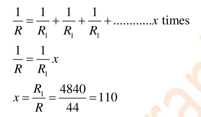
Therefore, 110 electric bulbs are connected in parallel.
