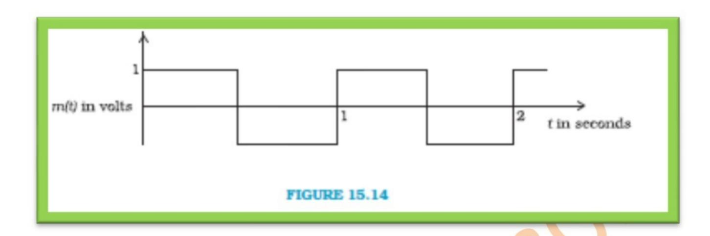
The carrier wave is given by  $c(t) = 2\sin(8\pi t)$  volts.
