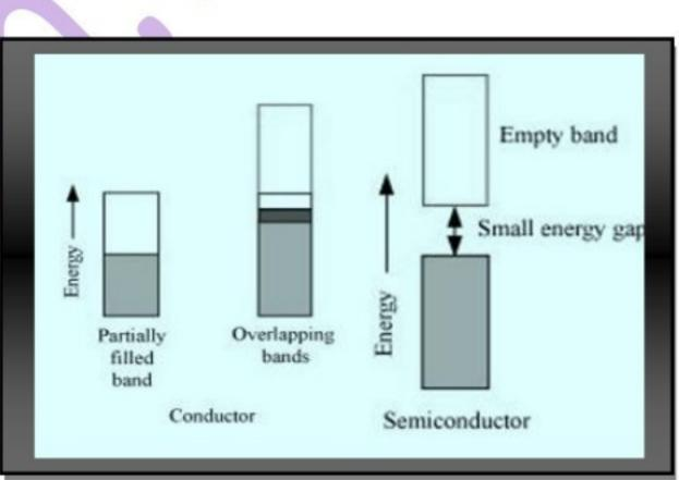
conduction band.Therefore, some electrons can jump easily from the valence band to the conduction band and conduct electricity.
