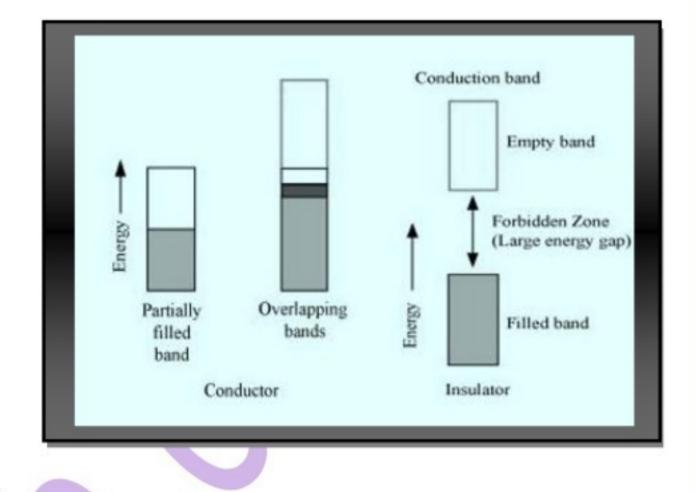
(ii)Conductor: - valence band of a conductor is partially-filled or it overlaps with a higher unoccupied band known as conduction band. Conduction band is higher energy level. So, the electrons can flow easily if we apply an electric field.
